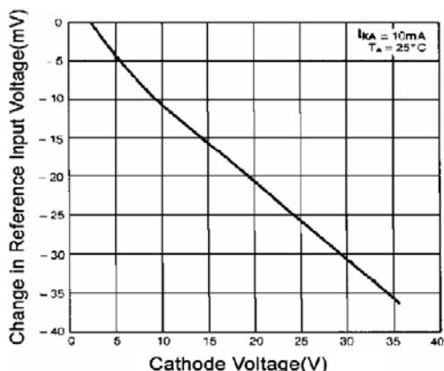
Change in Reference Input Voltage vs. Cathode Voltage
